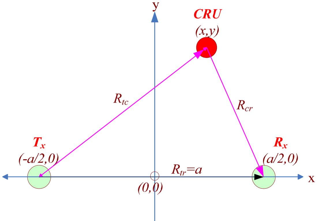
Fig. 5 Elliptic CRU operation scenario with movable CRU and fixed  $R_r (=a)$
