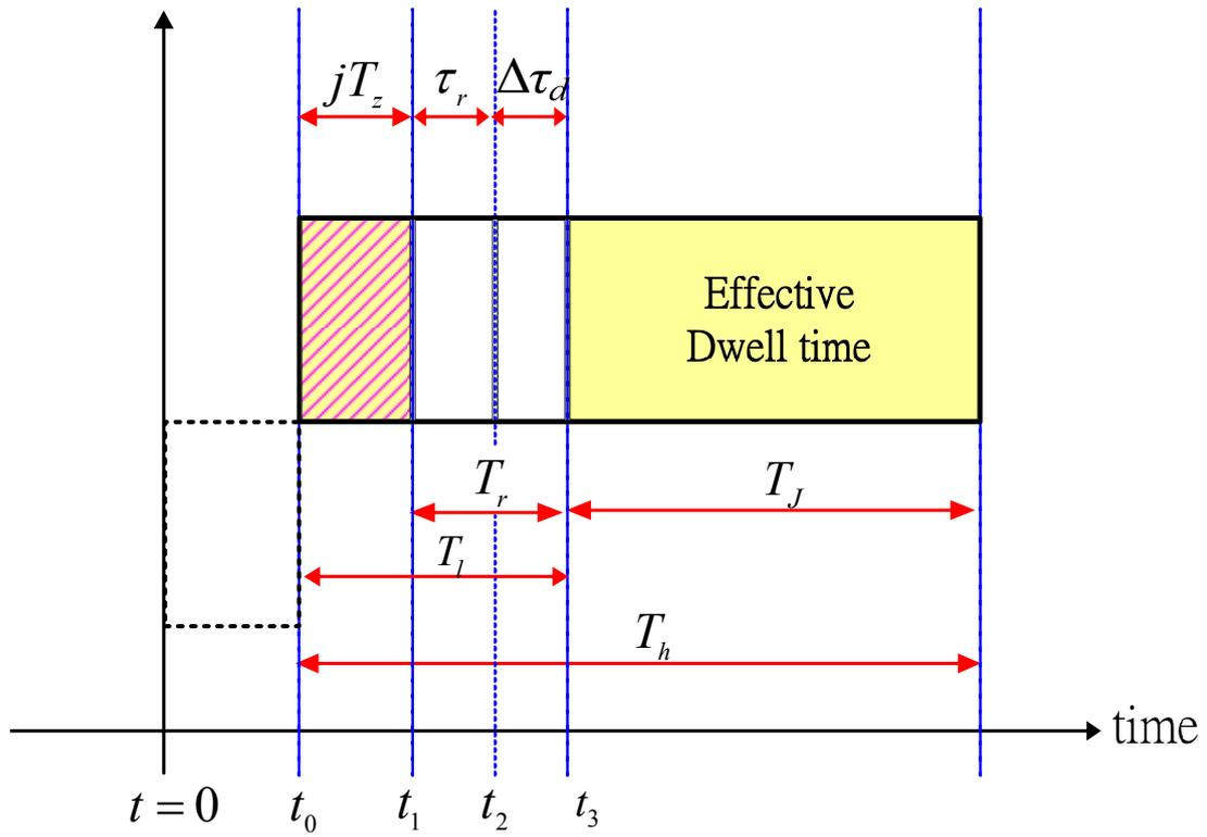
Fig. 3 Effective dwell time ( $T_J$ ) and latency time breakdown for CRU operation
