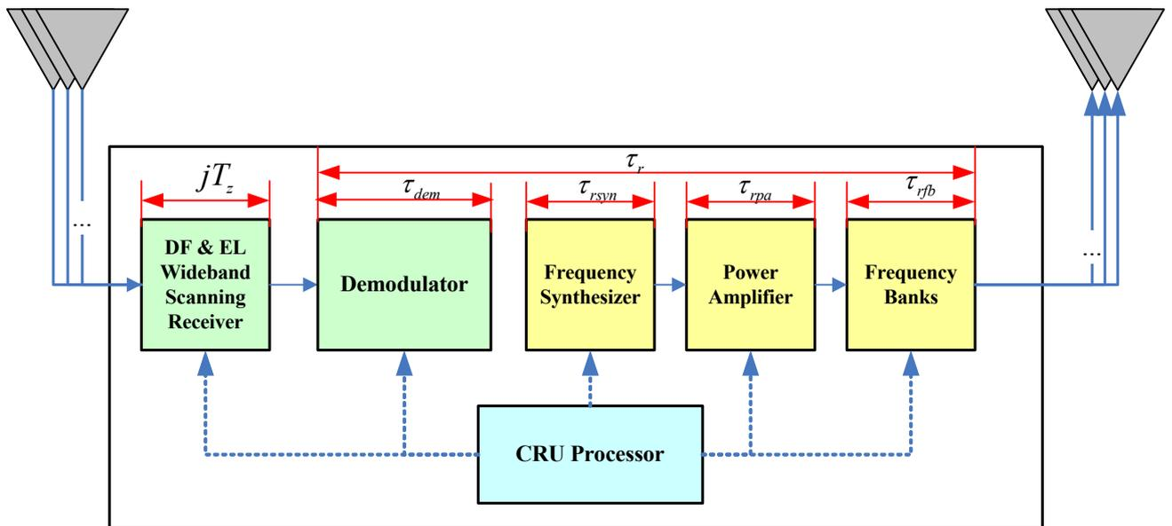
Fig. 2 Cognitive radio unit (CRU) architecture and latency time breakdown
